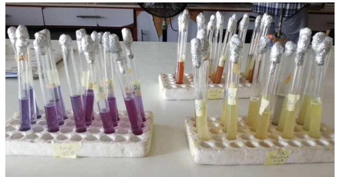
Figure 2 Presumptive test after incubation for 48 hours
